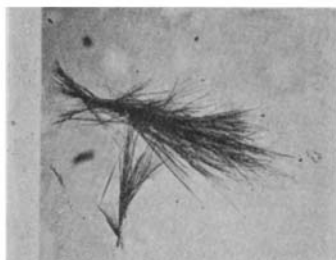
FIG. 3. Morphine (0.1 \mu\text{g.} ) with potassium cadmium iodide \times 50 .
